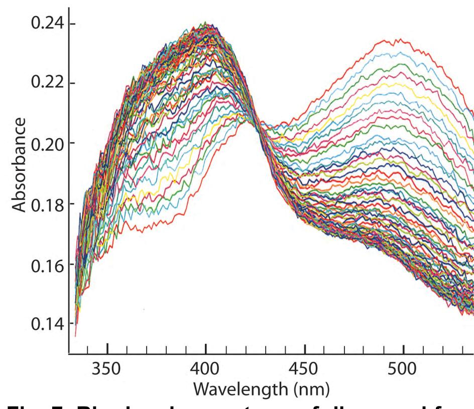
Fig. 7. Rhodopsin spectrum of dispersed frog retina within the integrating cavity absorption chamber. Scans: 40 sec at 2 scans/sec with exposure to 515 nm LED at 100 flashes/sec..
