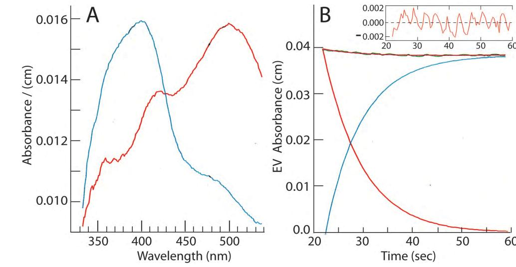
Fig. 8. Spectral analysis of Fig. 7 data set. Absorbance was corrected according to Javorfi et al (2006)<sup>6</sup>. A) Red, pre-bleach; blue, postbleach spectra. **B**) Data was fit to two species: A -> B with rate constant of 0.132 sec<sup>-1</sup>.
