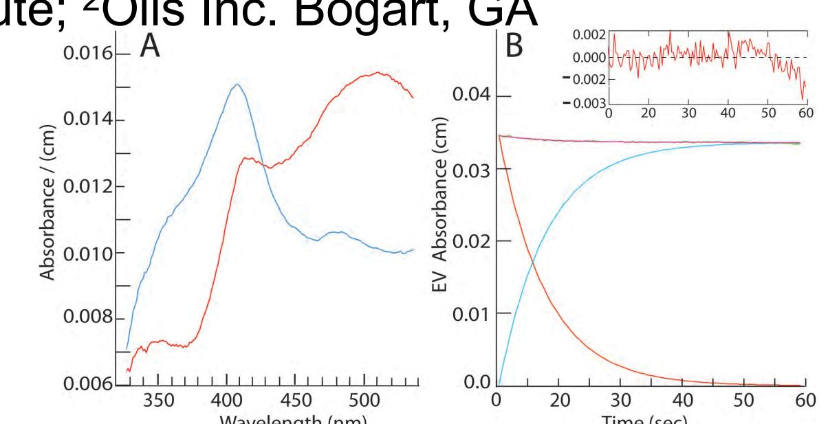
Fig. 9. Rhodopsin spectrum of a single intact frog retina. An intact neural retina was detached and transferred directly to the integrating cavity where it was exposed to 515 nm LED at 100 flashes/sec. Scans were taken for 40 sec at a rate of 2 scan/sec. Absorbance was corrected according to Javorfi et al (2006)<sup>6</sup> A) Red, pre-bleach; blue, post-bleach spectra. **B**) Data was fit: A -> B; rate = 0.105 sec<sup>-1</sup>.
