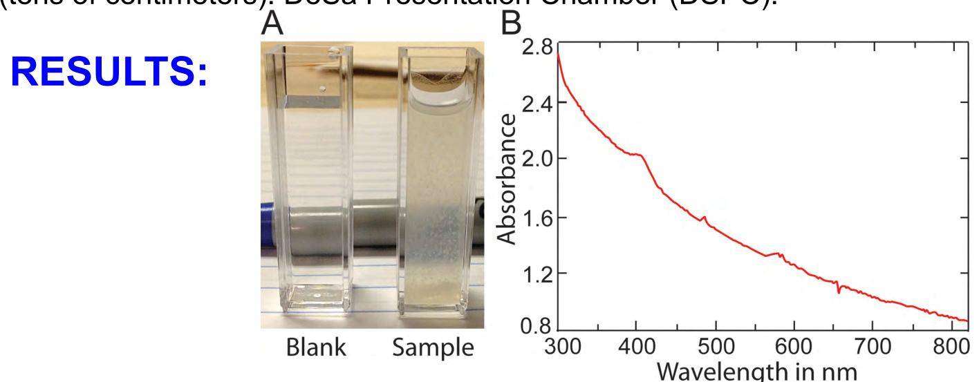
Fig 5. Conventional absorbance spectroscopy of a bleached crude outer segment suspension. A) Rectangular cuvette with buffer (blank); bleached outer segment preparation (sample). B) Absorbance spectrum obtained using a rectangular quartz cuvette in a HP 8452 diode array spectrophotometer. The absorbance is dominated by Rayleigh scattering.
