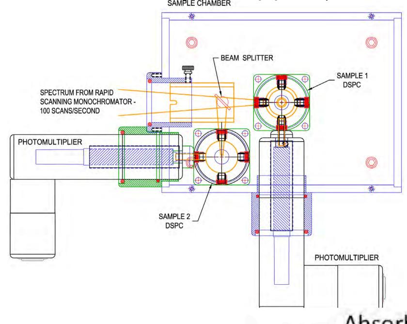
Fig 3. Diagram of the dual beam **CLARITY spectrophotometer**. This unit is equipped with an Olis rapid scaning UV / VIS mono-chrometer (RSM). The conventional single pass rectangular cuvette is replaced with a spherical cuvette, the DeSa Presentation Chamber (DSPC).
