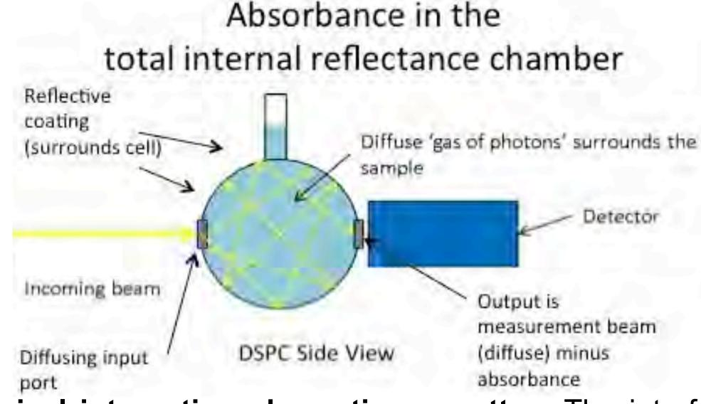
Spherical integrating absorption cuvette. The interference of light scattering is eliminated through the use of a spherical cuvette surrounded by a reflective material. The measurement beam is fully scattered (yellow lines). The effective path-length is markedly increased (tens of centimeters). DeSa Presentation Chamber (DSPC).
