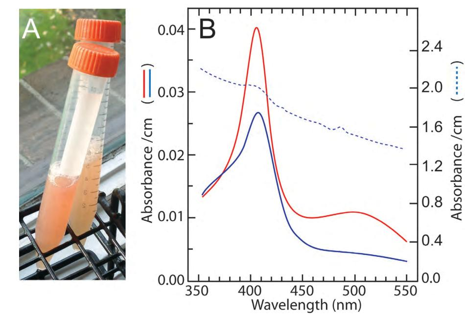
Fig 6. Rhodopsin spectra obtain using the integrating cavity absorption chamber. Crude outer segment suspension before (left) and after (right) bleaching. B) Absorbance spectra obtained before (red), and after (blue) bleaching under direct sunlight. Data from Fig 5 is superimposed (dashed line).
