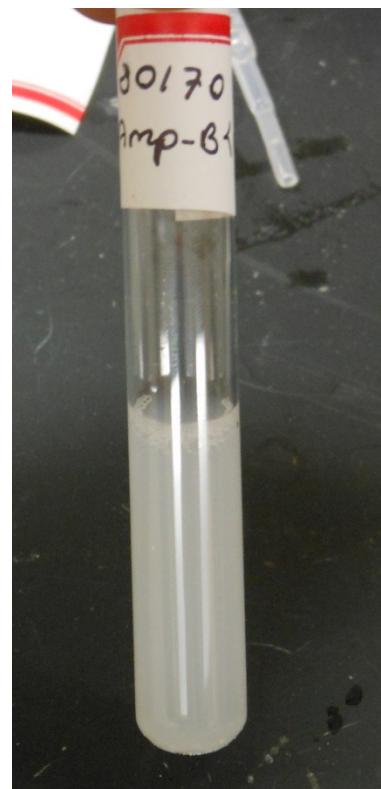
30-70 Peceol - Gelucire 44/14 with incorporated Amphotericin B in simulated gastric fluid on OLIS CLARITY 17
